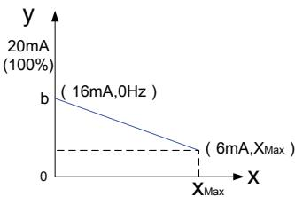
零偏  $b = y - kx = y (x=0 \text{ 时}) = 16 \text{ mA}$
